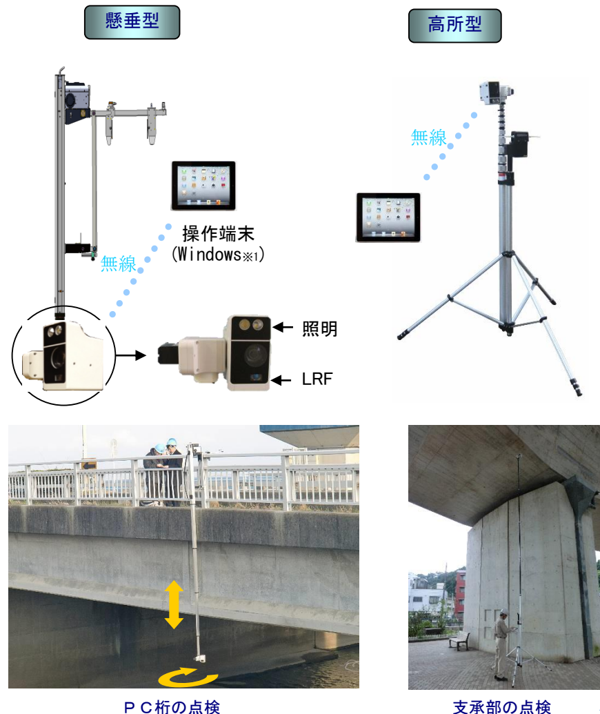
P C 桁の点検
